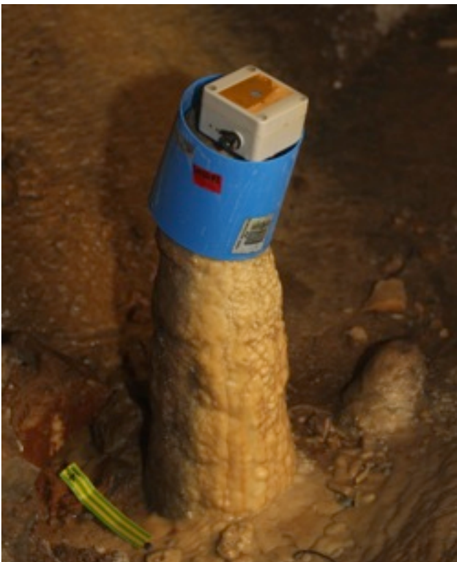
Above. Monitoring equipment in Harry Wood Cave Below. "Stalagmate" in place monitoring drip rates Photos: Steve Bourne
